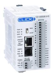
CLICK Ethernet Analog PLC, 24 VDC required, Ethernet and serial ports, Discrete Input: 4-point, DC, Analog Input: 4-channel, voltage, Discrete Output: 4-point, sourcing, Analog Output: 2-channel, voltage.
