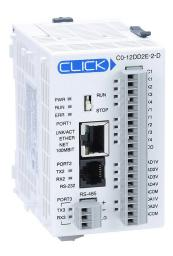
CLICK Ethernet Analog PLC, 24 VDC required, Ethernet and serial ports, Discrete Input: 4-point, DC, Analog Input: 4-channel, voltage, Discrete Output: 4-point, sourcing, Analog Output: 2-channel, voltage.
