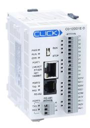
CLICK Ethernet Analog PLC, 24 VDC required, Ethernet and serial ports, Discrete Input: 4-point, DC, Analog Input: 2-channel, current/voltage, Discrete Output: 4-point, sinking, Analog Output: 2-channel, current/voltage.
