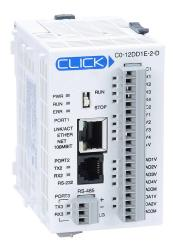
CLICK Ethernet Analog PLC, 24 VDC required, Ethernet and serial ports, Discrete Input: 4-point, DC, Analog Input: 4-channel, voltage, Discrete Output: 4-point, sinking, Analog Output: 2-channel, voltage.
