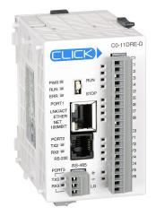
CLICK Ethernet Standard PLC, 24 VDC required, Ethernet and serial ports, Discrete Input: 8-point, DC, Discrete Output: 6-point, relay.
