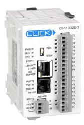
CLICK Ethernet Standard PLC, 24 VDC required, Ethernet and serial ports, Discrete Input: 8-point, DC, Discrete Output: 6-point, sourcing.
