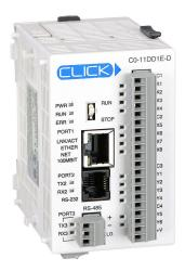
CLICK Ethernet Standard PLC, 24 VDC required, Ethernet and serial ports, Discrete Input: 8-point, DC, Discrete Output: 6-point, sinking.
