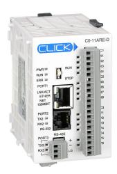
CLICK Ethernet Standard PLC, 24 VDC required, Ethernet and serial ports, Discrete Input: 8-point, AC, Discrete Output: 6-point, relay.
