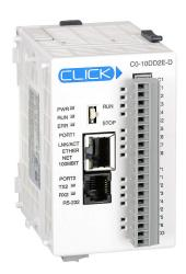
CLICK Ethernet Basic PLC, 24 VDC required, Ethernet and serial ports, Discrete Input: 8-point, DC, Discrete Output: 6-point, sourcing.
