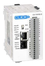
CLICK Ethernet Basic PLC, 24 VDC required, Ethernet and serial ports, Discrete Input: 8-point, AC, Discrete Output: 6-point, relay.
