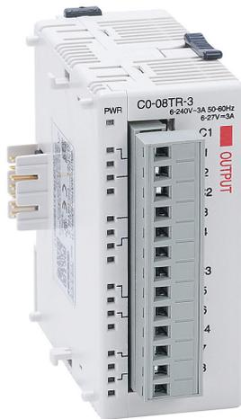
CLICK relay output module, 8-point, 6-27 VDC/6-240 VAC, (8) Form A (SPST) no-suppression, 4 isolated common(s), 2 point(s) per common, 3A/point. Removable terminal block included.
