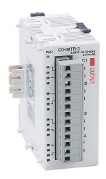
CLICK relay output module, 8-point, 6-27 VDC/6-240 VAC, (8) Form A (SPST) no-suppression, 4 isolated common(s), 2 point(s) per common, 3A/point. Removable terminal block included.
