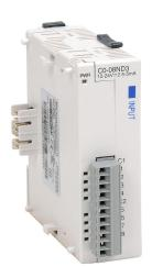
CLICK discrete input module, 8-point, 12-24 VDC, sinking/sourcing, 2 isolated common(s), 4 point(s) per common. Removable terminal block included.
