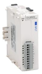
CLICK discrete input module, 8-point, 12-24 VDC, sinking/ sourcing, 2 isolated common(s), 4 point(s) per common. Removable terminal block included.
