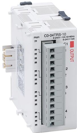
CLICK relay output module, 4-point, 6-24 VDC/6-240 VAC, (4) Form A (SPST) no-suppression, 4 isolated common(s), 1 point(s) per common, 10A/point. Removable terminal block included.
