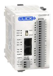
CLICK Standard PLC, 24 VDC required, serial ports, Discrete Input: 8-point, DC, Discrete Output: 6-point, sinking.
