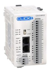
CLICK Standard PLC, 24 VDC required, serial ports, Discrete Input: 8-point, AC, Discrete Output: 6-point, relay.
