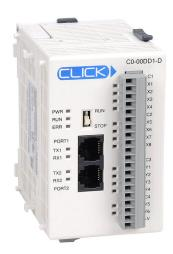
CLICK Basic PLC, 24 VDC required, serial ports, Discrete Input: 8-point, DC, Discrete Output: 6-point, sinking.
