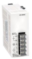
CLICK AC power supply, 100-240 VAC nominal input, 24 VDC nominal output, 0.5A continuous.
