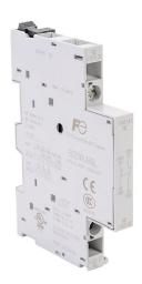
Fuji Electric auxiliary contact, left side mount, (2) N.C. contact(s), 6A @ 120 VAC/1.1A @ 120 VDC. For use with BM3R/BM3V series manual motor protector.
