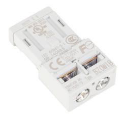
Fuji Electric auxiliary contact, front mount, (1) N.C. contact(s), 1.5A @ 230VAC/0.55A @ 110VDC. For use with BM3R/BM3V series manual motor protector.
