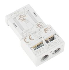
Fuji Electric auxiliary contact, front mount, (1) N.O. contact(s), 1.5A @ 230VAC/0.55A @ 110VDC. For use with BM3R/BM3V series manual motor protector.
