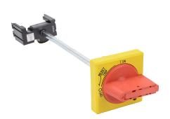
Fuji Electric rotary handle, selector, red/yellow, external front mount, 2-position, lockable in OFF only, defeatable. For use with BM3V series manual motor protector. Handle, shaft, operator, and mounting screws included.
