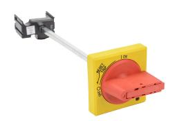
Fuji Electric rotary handle, selector, red/yellow, external front mount, 2-position, lockable in OFF only, defeatable. For use with BM3RH series manual motor protector. Shaft, operator, and mounting screws included.
