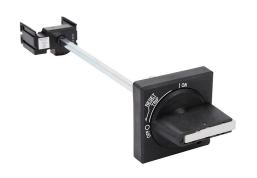
Fuji Electric rotary handle, selector, black, external front mount, 2-position, lockable in OFF only, defeatable. For use with BM3RH series manual motor protector. Handle, shaft, operator, and mounting screws included.
