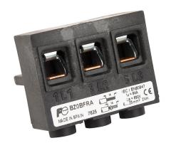
Fuji Electric incoming power terminal block, maximum current 64A, maximum wire size 4AWG. For use with BM3RH busbars. For incoming power to busbar system.
