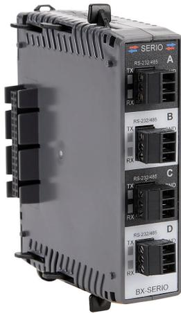
BRX communication module, Do-more protocol, Modbus RTU and ASCII, 4 ports, buffered, (4) RS-232/RS-485 (3-pin terminal) port(s). For use with all BRX PLCs. (4) BX-RTB03S terminal blocks included.
