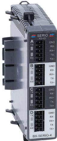
BRX communication module, Do-more protocol, Modbus RTU and ASCII, 4 ports, buffered, (4) RS-422 (5-pin terminal) port(s). For use with all BRX MPUs. (4) BX-RTB05S terminal blocks included.
