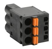
BRX terminal block kit, 180-degree spring clamp, replacement. For use with BRX 18-point PLCs. Includes (1) 3-pin 5mm terminal block.
