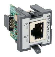
BRX communication POM module, Sparkplug B, 1 port, (1) Ethernet 10/100Base-T (RJ45) port(s). For use with all BRX MPUs. Requires 3rd party Sparkplug B compliant MQTT broker.
