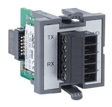
BRX communication POM module, Do-more protocol, Modbus RTU and ASCII, 1 port, buffered, (1) RS-422 (5-pin terminal) port(s). For use with all BRX MPUs. BX-RTB05S terminal block included.
