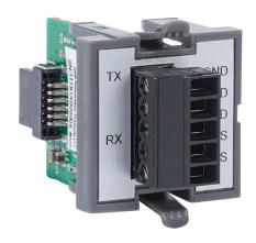
BRX communication POM module, Do-more protocol, Modbus RTU and ASCII, 1 port, buffered, (1) RS-232 (5-pin terminal) port(s). For use with all BRX MPUs. BX-RTB05S terminal block included.
