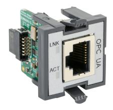
BRX communication POM module, OPC-UA, 1 port, (1) Ethernet 10/100Base-T (RJ45) port(s). For use with all BRX MPUs.
