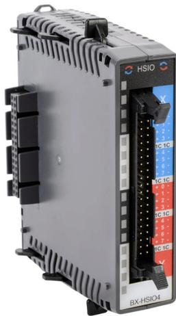
BRX pulse combo module, 2 MHz maximum switching frequency, 8 high-speed input point(s), sinking/sourcing/TTL, differential and single-ended encoder input(s), 8 high-speed output point(s), sinking/sourcing/TTL, differential and single-ended output(s).
