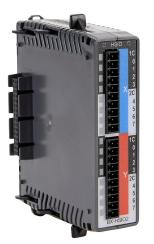
BRX pulse combo module, 250 kHz maximum switching frequency, 8 high-speed input point(s), sinking/sourcing, single-ended encoder input(s), 8 high-speed output point(s), sourcing, single-ended output(s).
