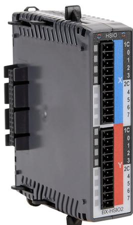
BRX pulse combo module, 250 kHz maximum switching frequency, 8 high-speed input point(s), sinking/sourcing, single-ended encoder input(s), 8 high-speed output point(s), sourcing, single-ended output(s).
