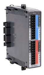
BRX pulse combo module, 250 kHz maximum switching frequency, 8 high-speed input point(s), sinking/sourcing, single-ended encoder input(s), 8 high-speed output point(s), sinking, single-ended output(s).
