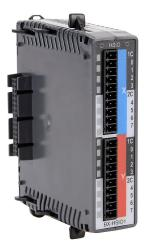
BRX pulse combo module, 250 kHz maximum switching frequency, 8 high-speed input point(s), sinking/sourcing, single-ended encoder input(s), 8 high-speed output point(s), sinking, single-ended output(s).
