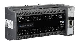
BRX Do-more PLC, 120-240 VAC required, Ethernet and serial ports, microSD card slot, Discrete Input: 20-point, AC/DC, Analog Input: 4-channel, current/voltage, Discrete Output: 16-point, relay, Analog Output: 2-channel, current/voltage.
