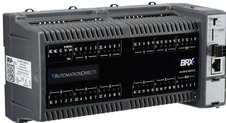
BRX Do-more PLC, 12-24 VDC required, Ethernet and serial ports, microSD card slot, Discrete Input: 20-point, AC/DC, Analog Input: 4-channel, current/voltage, Discrete Output: 16-point, relay, Analog Output: 2-channel, current/voltage.
