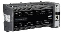
BRX Do-more PLC, 12-24 VDC required, Ethernet and serial ports, microSD card slot, Discrete Input: 20-point, AC/DC, Analog Input: 4-channel, current/voltage, Discrete Output: 16-point, sourcing, Analog Output: 2-channel, current/voltage.
