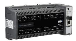
BRX Do-more PLC, 120-240 VAC required, Ethernet and serial ports, microSD card slot, Discrete Input: 20-point, AC/DC, Analog Input: 4-channel, current/voltage, Discrete Output: 16-point, sinking, Analog Output: 2-channel, current/voltage.
