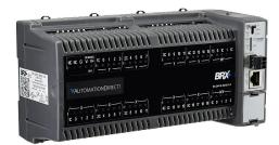
BRX Do-more PLC, 12-24 VDC required, Ethernet and serial ports, microSD card slot, Discrete Input: 20-point, AC/DC, Analog Input: 4-channel, current/voltage, Discrete Output: 16-point, sinking, Analog Output: 2-channel, current/voltage.
