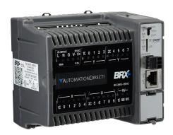
BRX Do-more PLC, 120-240 VAC required, Ethernet and serial ports, microSD card slot, Discrete Input: 10-point, AC/DC, Analog Input: 1-channel, current/voltage, Discrete Output: 8-point, relay, Analog Output: 1-channel, current/voltage.
