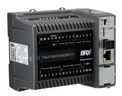
BRX Do-more PLC, 12-24 VDC required, Ethernet and serial ports, microSD card slot, Discrete Input: 10-point, AC/DC, Analog Input: 1-channel, current/voltage, Discrete Output: 8-point, sourcing, Analog Output: 1-channel, current/voltage.
