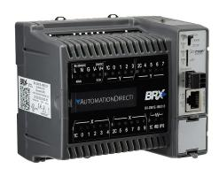
BRX Do-more PLC, 120-240 VAC required, Ethernet and serial ports, microSD card slot, Discrete Input: 10-point, AC/DC, Analog Input: 1-channel, current/voltage, Discrete Output: 8-point, sinking, Analog Output: 1-channel, current/voltage.
