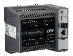
BRX Do-more PLC, 12-24 VDC required, Ethernet and serial ports, microSD card slot, Discrete Input: 10-point, AC/DC, Analog Input: 1-channel, current/voltage, Discrete Output: 8-point, sinking, Analog Output: 1-channel, current/voltage.
