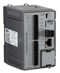
BRX Do-more PLC, 12-24 VDC required, Ethernet and serial ports, microSD card slot, Discrete Input: 6-point, AC/DC, Analog Input: 1-channel, current/voltage, Discrete Output: 4-point, relay, Analog Output: 1-channel, current/voltage.
