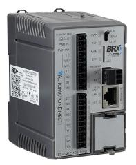
BRX Do-more PLC, 12-24 VDC required, Ethernet and serial ports, microSD card slot, Discrete Input: 6-point, AC/DC, Analog Input: 1-channel, current/voltage, Discrete Output: 4-point, sourcing, Analog Output: 1-channel, current/voltage.
