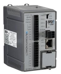
BRX Do-more PLC, 12-24 VDC required, Ethernet and serial ports, microSD card slot, Discrete Input: 6-point, AC/DC, Analog Input: 1-channel, current/voltage, Discrete Output: 4-point, sinking, Analog Output: 1-channel, current/voltage.
