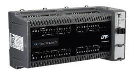
BRX Do-more PLC, 12-24 VDC required, serial port, microSD card slot, Discrete Input: 20-point, AC/DC, Discrete Output: 16-point, sourcing.
