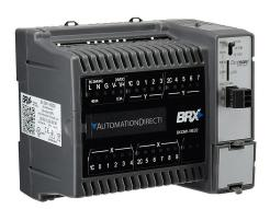
BRX Do-more PLC, 120-240 VAC required, serial port, microSD card slot, Discrete Input: 10-point, AC/DC, Discrete Output: 8-point, sourcing.
