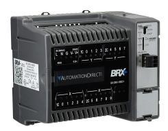
BRX Do-more PLC, 120-240 VAC required, serial port, microSD card slot, Discrete Input: 10-point, AC/DC, Discrete Output: 8-point, sinking.
