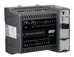
BRX Do-more PLC, 120-240 VAC required, serial port, microSD card slot, Discrete Input: 10-point, AC, Discrete Output: 8-point, relay.
