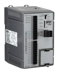
BRX Do-more PLC, 12-24 VDC required, serial port, microSD card slot, Discrete Input: 6-point, AC/DC, Discrete Output: 4-point, sourcing.
